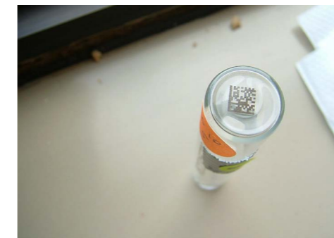
Figure 3.2.3-1 GS1 DataMatrix Laser symbol
