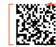
Figure 3.6.1.2-5 Fixed Pattern Damage
