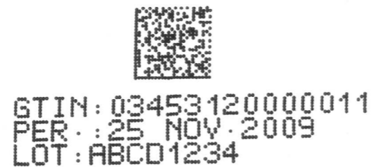
Figure 3.2.2-1 Inkjet printed GS1 DataMatrix
