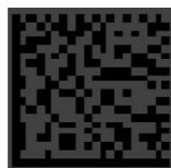
Figure 3.6.1.2-1 A symbol with very poor Symbol Contrast.
