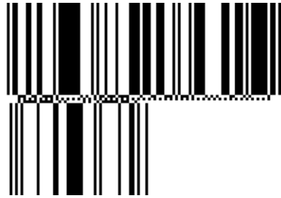
Figure A1.3 – 1. Example of GS1 DataBar Expanded Stacked Bar Code that uses concatenation
