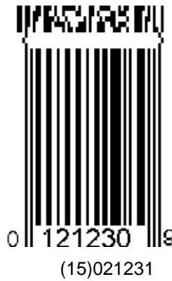
Figure A1.3 - 2 Example of mixed GS1 Symbologies (GTIN encoded in UPC-E, Best Before Date in Composite)
