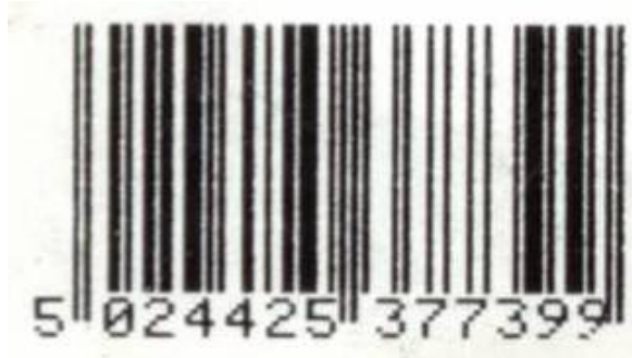
Figure 5.5.3.3.12 – 1. Symbol with Edge Determination Problem
